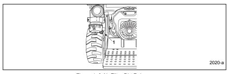
Figure 4-3 Air Filter Dirt Release
